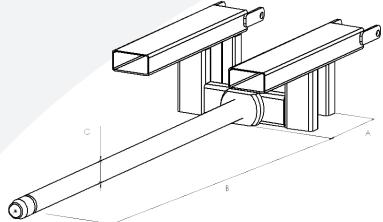
We manufacture our forklift booms to order to ensure the roll diameter and under-slung nature of the design does not cause any conflict with your forklift truck forks..
